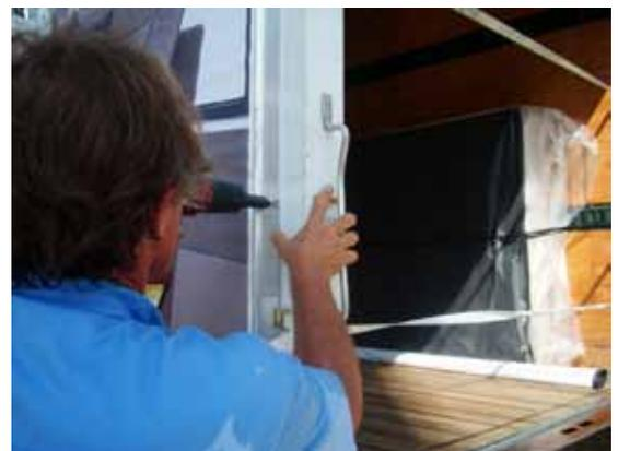
**8** Slide the conduit rods into the bottom pole pocket of the TruckSkin. At this point, note all fuel filler necks, mud flaps and step bumpers which are in the way. These obstacles may need to be notched out on the TruckSkin, so mark them now.
