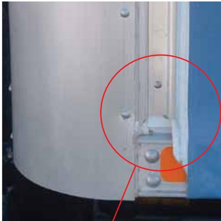
Correct placement of bottom of front rail of a Supreme body.
