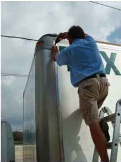
NOTE: You must leave a 2 inch gap between the front vertical rail and the top horizontal rail for the graphics to slide into. The gap can be on either the front or top rail.
