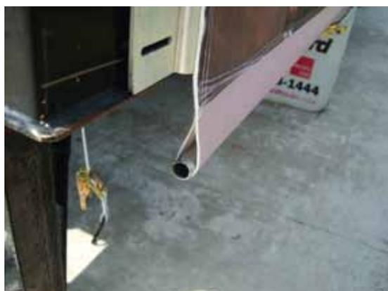
One of the conduit pieces will need to be cut to fit. You may also need to cut out sections to go around gas caps, mud flaps or tires if there is not ample clearance (6") between the tire and truck body.
