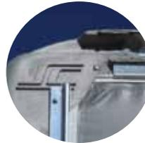
Type 1: Begin at bottom line under the logo. The front rail extends down over the rivet line towards the rear of the body, then finishes above the bottom rail 1 1/2" so that the sign does not get pinched.
